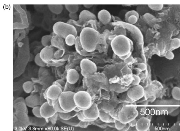
Fig. 10. (a) XRD analysis, and (b) FEGSEM image of particulate iron carbide, produced by treatment of pure magnetite powder with hydrogen and acetylene.
